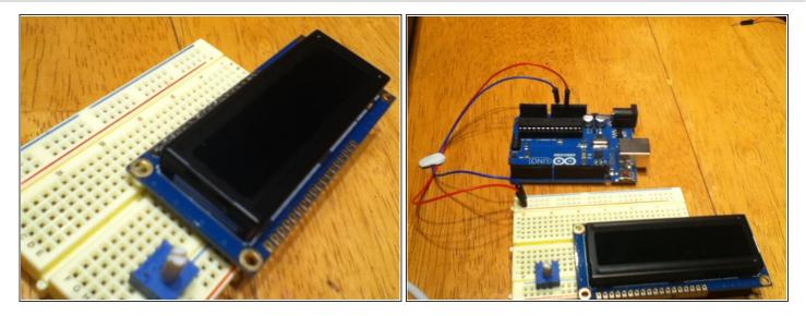
Now we will prepare everything to start connecting to the Arduino. Insert the display into the breadboard with the pot next to it. Then connect 5V and GND to the breadboard rails as I have done. Good.
